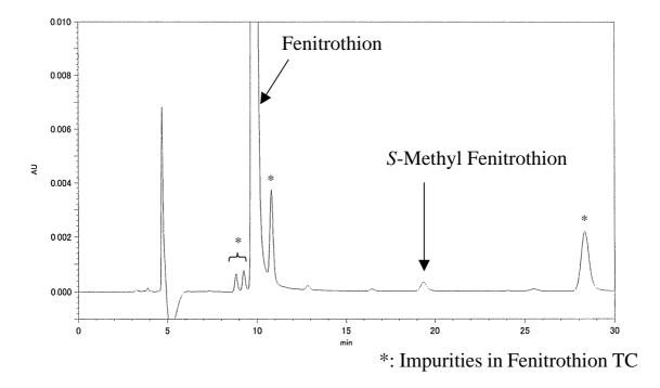
Fig.3 Example of Chromatogram of S-Methyl Fenitrothion
